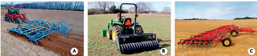
Figure 14.2. Soil cultivation equipment: A) cultivator, B) cultipacker, C) set of harrows
